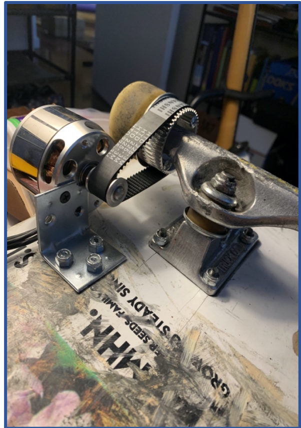
Initial motor mounting on skateboard
