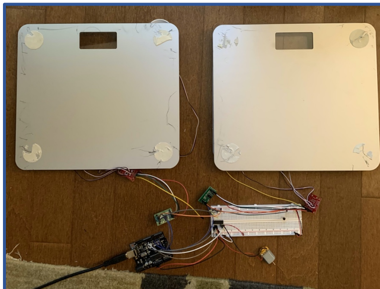
Running a small DC motor by reading weight distribution across two scales. Determine motor rotation direction and speed with H-Bridge IC chip.
